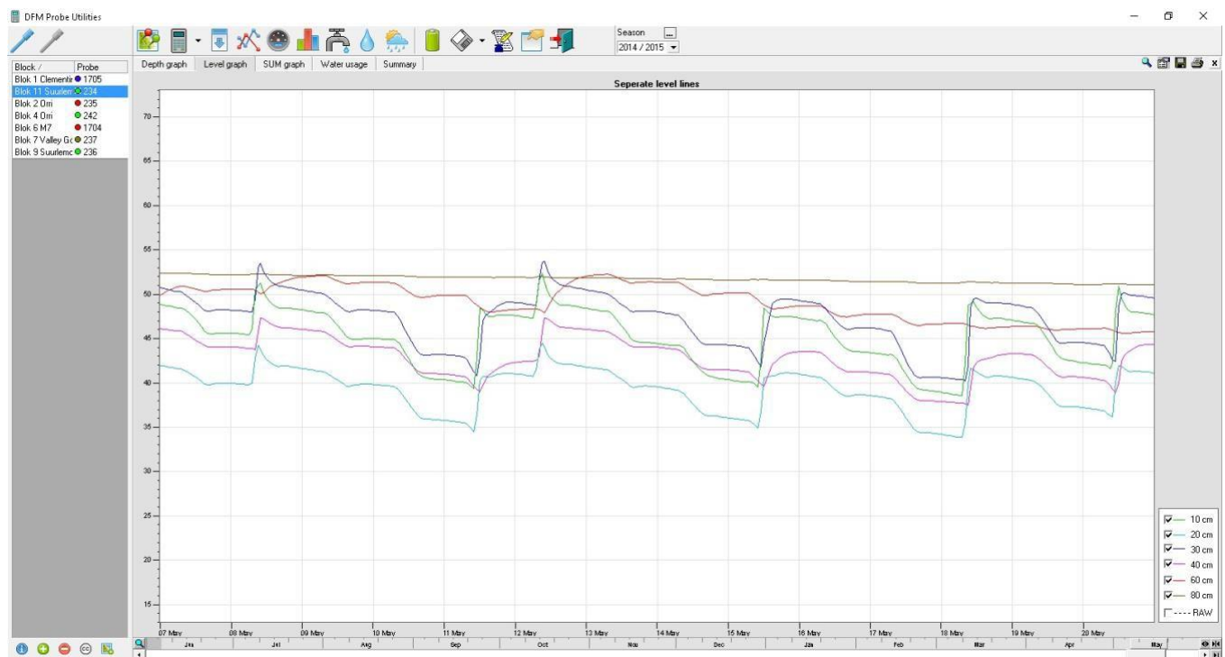
Figure 2. DFM probe utilities measurements showing water withdrawals at 20, 40 & 60 cm – Block 11 Lemons
